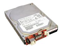
3. Using the provided Y-power cable, connect the 4-pin floppy connector to the power connector of the converter. This will provide power to the converter.
